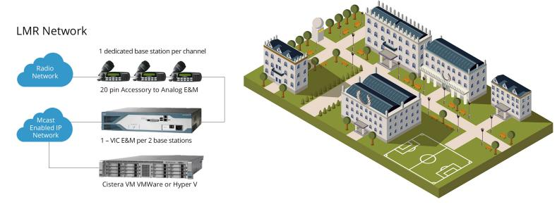
This diagram shows the components of the LMR recording setup including base stations for each monitored channel, Cisco ISR and the Cistera VM platform. Refer to configuration guide for additional details.
